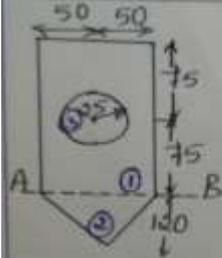
Moment of Inertia of shaded area about AB } MI of fig ① + MI of fig ② - MI of fig ③
