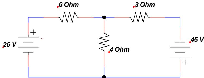
Assuming loop current in clockwise direction  $I_1$  in loop 1 ,And  $I_2$  in loop2
