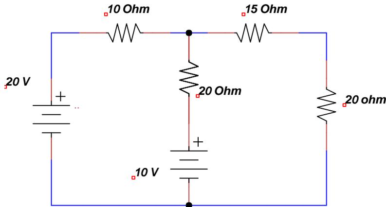
Assuming loop current in clockwise direction  $I_1$  in loop 1 ,And  $I_2$  in loop2
